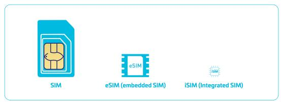
An eSIM occupies x60 less space than a nano SIM. Furthermore, iSIM occupies no space as it is part of the cellular modem chipset.
