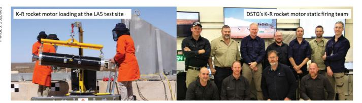
rocket motors, including the 10-inch (254mm) diameter Koonibba-Rising (K-R) class rocket motor. K-R was demonstrated in September 2023 at Woomera and it represents the largest advanced, military-relevant SRM designed and produced in-country to date.
