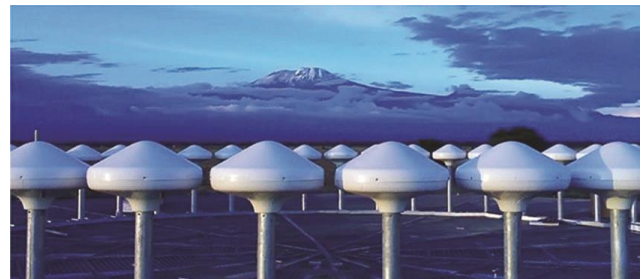
Doppler VHF Omnidirectional Radio ranging system DVOR 532 (Credit: Thales)
