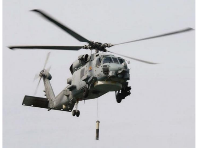
A US Navy MH-60R Seahawk with a Thales dipping sonar (credit – LM)
