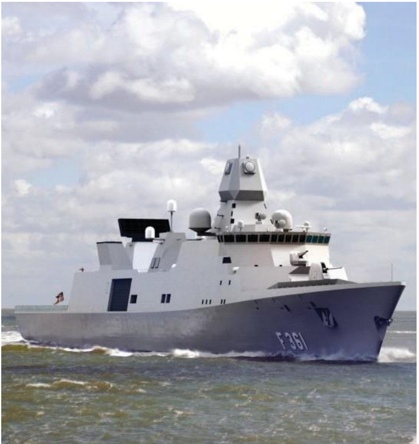
HMS Iver Huitfeldt with Thales APAR multifunction radar and Thales SMART-L volume search radar (credit – Thales Group)
