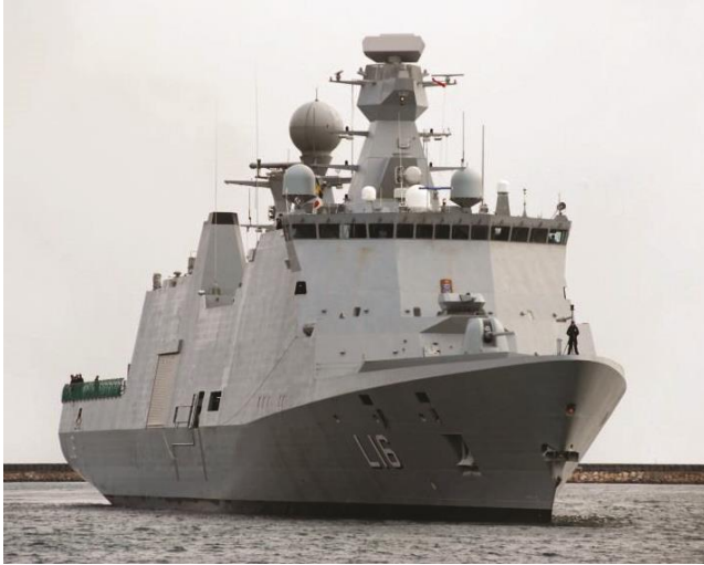
HMS Absalon with the Thales SMART-S Mk2 surveillance radar (credit – Thales Group)
